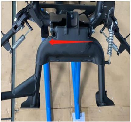
A photograph showing the main stand assembly from a wider perspective. A red arrow points to the main stand axis, which is the central vertical support.                   |
