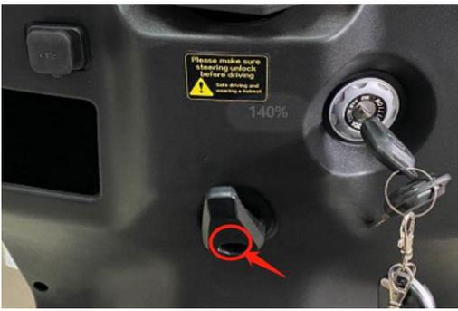
A close-up photograph of the steering lock assembly on a vehicle. A red circle highlights a bolt on the lock cover. A key is inserted into the lock cylinder. A yellow warning sticker is visible above the lock, and the text '140%' is printed on the plastic housing. |
