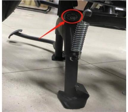
A close-up photograph of the main stand assembly, similar to the first image. A red circle highlights the sub spring mechanism, and a red arrow points to it from the left. |
