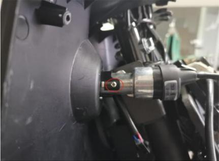
A close-up photograph showing a cross screwdriver being used to remove a screw from the lock cover. A red circle highlights the screw head.                                                                                                                   |
