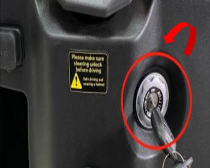
A close-up photograph of the steering lock assembly. A red circle highlights the lock cover, and a red curved arrow indicates it should be turned to the left. A key is inserted into the lock cylinder. A yellow warning sticker is visible above the lock. |
