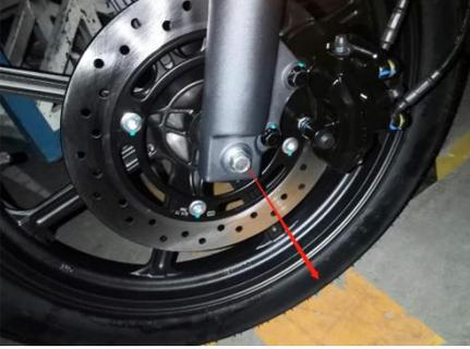
A photograph of the front wheel assembly. A red arrow points to the axle, indicating the direction to pull it out. The wheel is mounted on the motorcycle's fork, and a disc brake rotor is visible.        |
